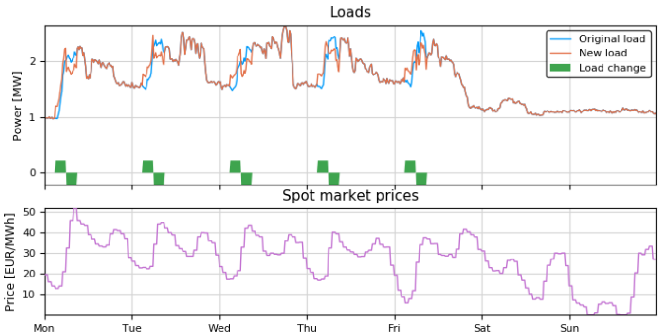
Figure 42: Illustration of flexibility activation of a Styrian load for week 24 of the year 2013.
